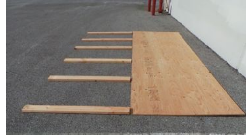
3/4 inch plywood & 2x4 supports
