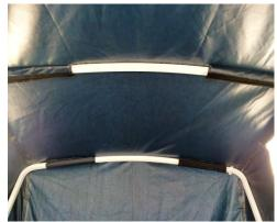
11. Attach the velcro along the full length front cross bar pole resting on the ground.
