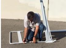
5. Use the four bolts and wing nuts (attached to the vertical poles) to attach the two vertical support poles to the frame.
